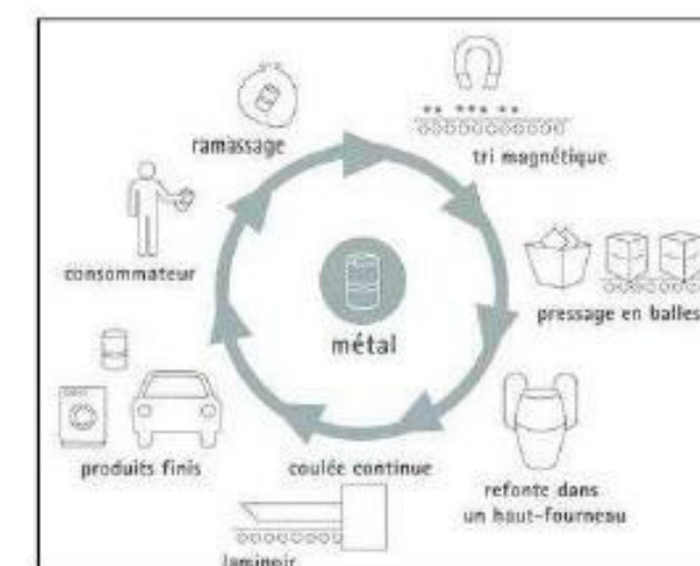
Figure 31: Recyclage des structures porteuses
