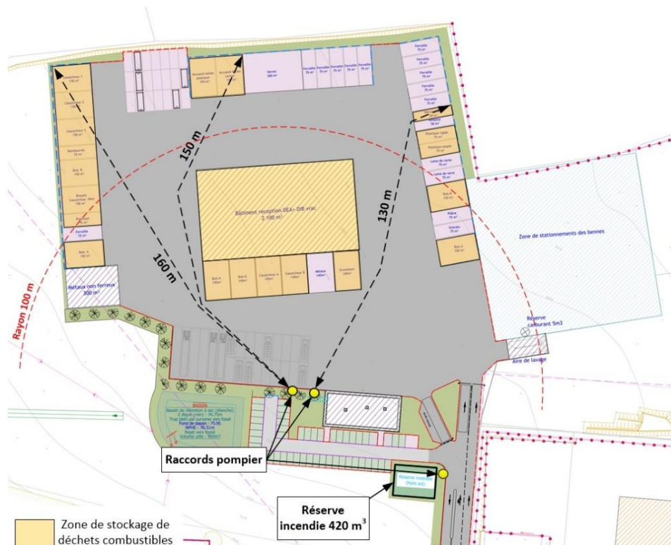
Figure n°3. Points raccord pompier
