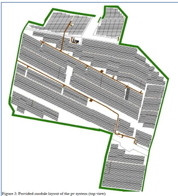
Figure 2: Provided module layout of the pv system (top view)
